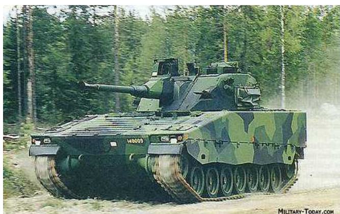
Fast, carries troops, but not a tank. Armour is "only" against 30mm tops, but CV90 can be fitted with reactive armour against shaped charges.
