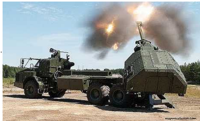
Archer fires up to 9 rounds/min, up to 60 km with Excalibur GPS ammo, said to hit within 5 metres of target!
