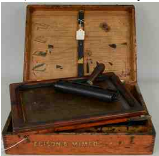
An early Edison mimeograph. The roller is used over a paper in the inked frame.
