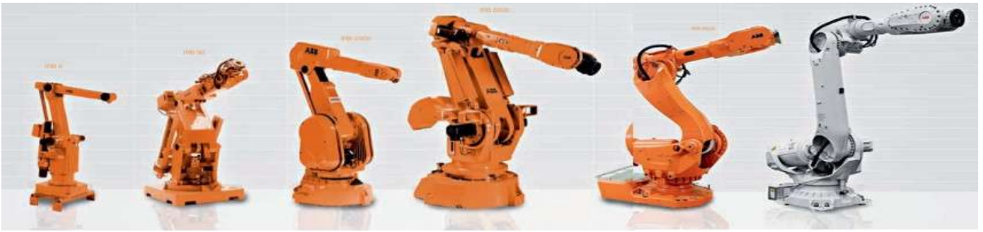
IRB6 far left claims to be the world's first electric, CPU controlled industrial robot. Here its evolution. See https://library.e.abb.com/public/c1ecdae9855e5452c1257d200053f273/24-31%202m433_EN_72dpi.pdf
