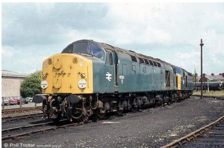
*[[The distinctive "whistle" of the class 40 was the sound of the turbochargers going, which were well needed - by 1976 these locomotives were underpowered compared to subsequent diesel-electrics. The most famous, or infamous Class 40 was D326 (later renumbered 40 126) - some railwaymen considered it jinxed because of a couple of accidents and mechanical failures. It's best known as the loco which was the target of the Great Train Robbery in 1963. Wikipedia adds:*
