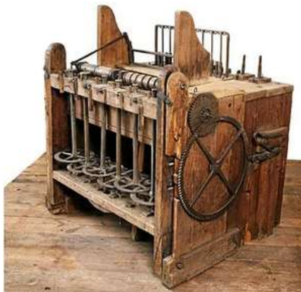
A machine for making cogwheels invented by Polhem.
