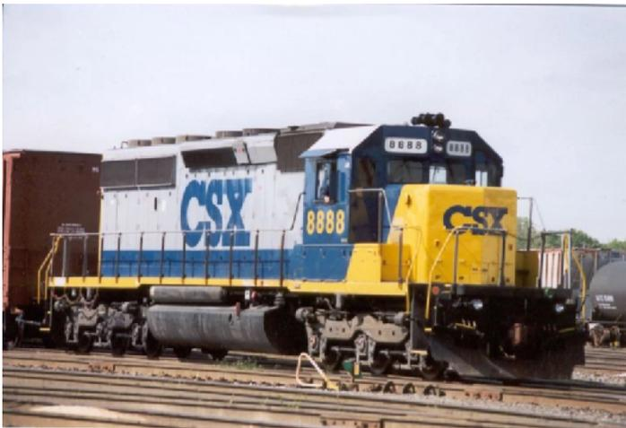
For the wholly or partially un-anoraked among you, braking on a train isn't quite like just stomping on a pedal. Dynamic braking, as employed on diesel and diesel-electric locos, uses the traction motor as a generator for the onboard brakes, but since these aren't enough to completely slow the engine, air brakes are used in concert, both those on the loco itself and the rest of the train.
